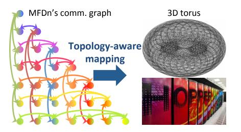
Topology-aware mapping of processes to the physical processors becomes more important as the gap between computational power and bandwidth widens. Communication groups are optimized through a column-major ordering of processes on the triangular grid [1].
