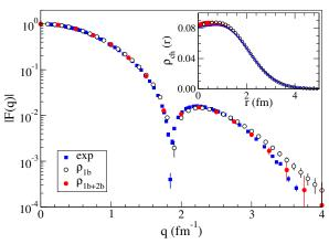
Longitudinal form factor: Two body terms in the density operator bring theoretical prediction closer to experimental data in the highmomentum transfer tail (q).
