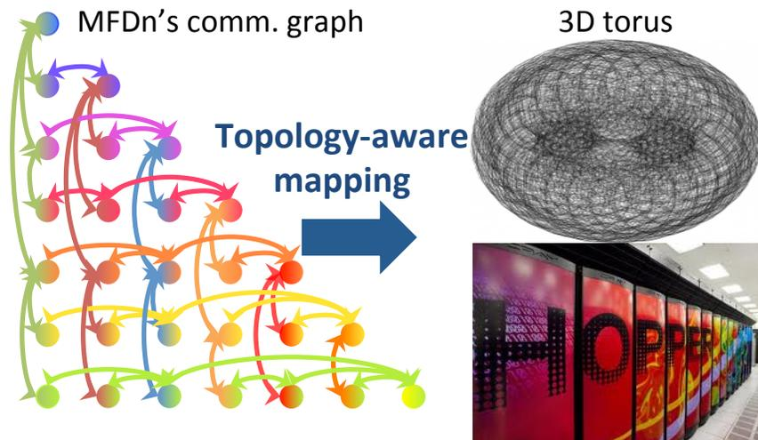
Topology-aware mapping of processes to the physical processors becomes more important as the gap between computational power and bandwidth widens. Communication groups are optimized through a column-major ordering of processes on the triangular grid [1].
