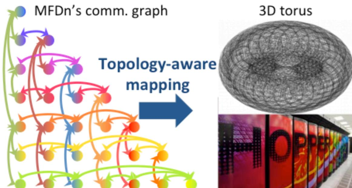
Topology-aware mapping of processes to the physical processors becomes more important as the gap between computational power and bandwidth widens. Communication groups are optimized through a column-major ordering of processes on the triangular grid [1].
